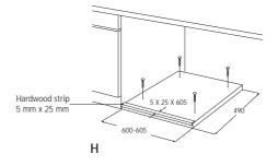
With the appliance installed adjust all four feet ensuring the machine is stable, and a clearance of approximately 5 mm is left between the top of the machine and the underside of the worktop.
